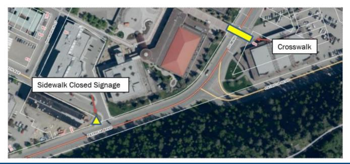
In the following example, pedestrian signage was done well. Signs notifying vehicular and pedestrian traffic of upcoming construction was given at the crosswalk immediately preceding the sidewalk closure allowing pedestrians opportunity to safely cross 15<sup>th</sup> Avenue at a marked pedestrian crossing.
