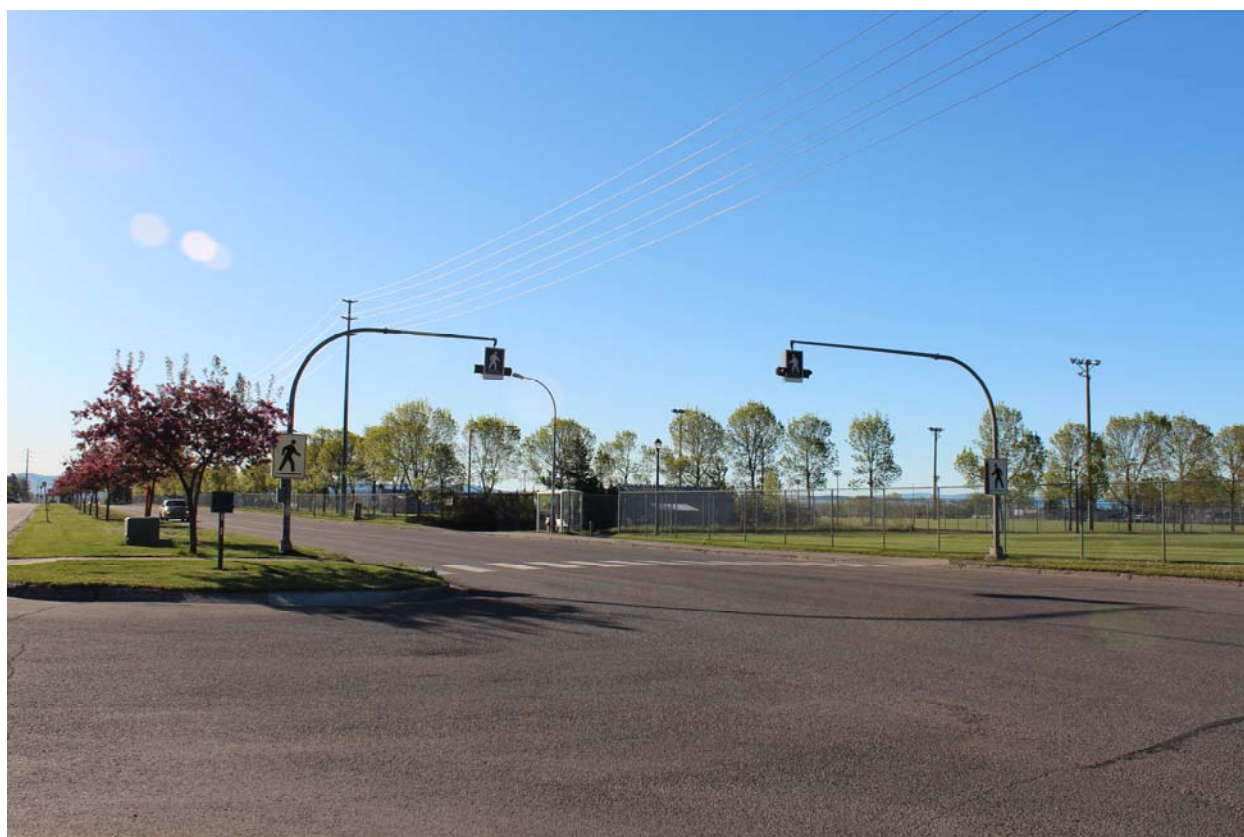
Figure 1: Overhead Flashing Beacon (OF) or Special Crosswalk – 15 th Avenue at Jarvis Street
