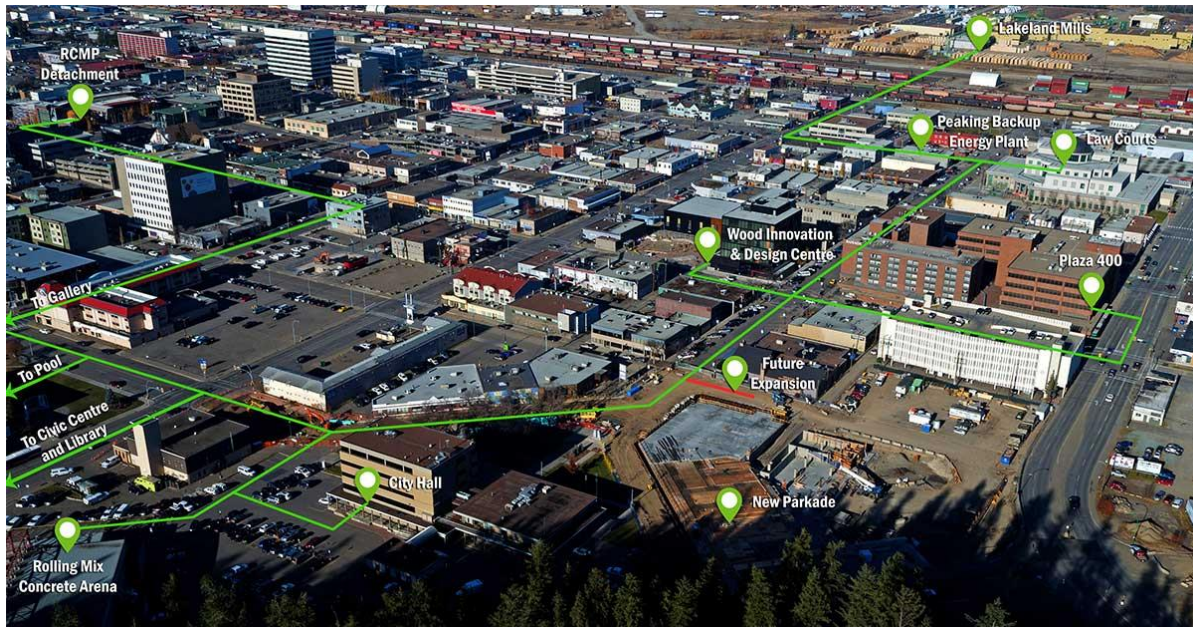
Prince George Downtown Renewable Energy System with current connections in green and future expansion indicated in red (Source: City of Prince George website).
