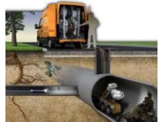
7km of Pipe Inspected Using a CCTV Camera
