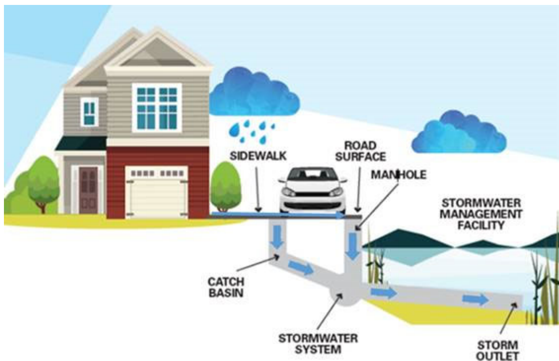
Figure 2: Typical Municipal Stormwater System
