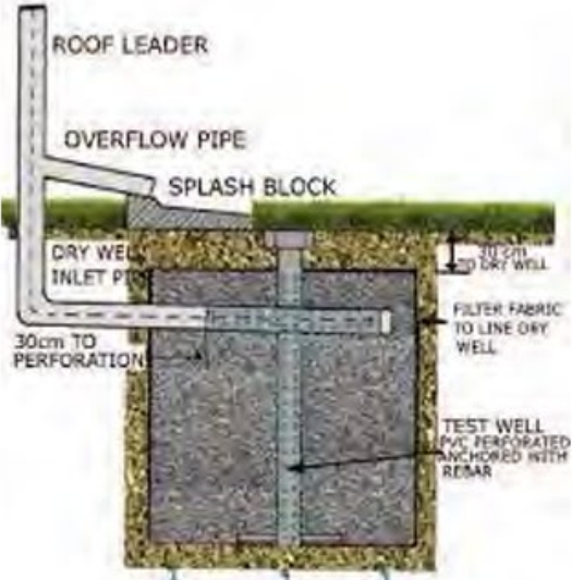
Soak Away Pit
