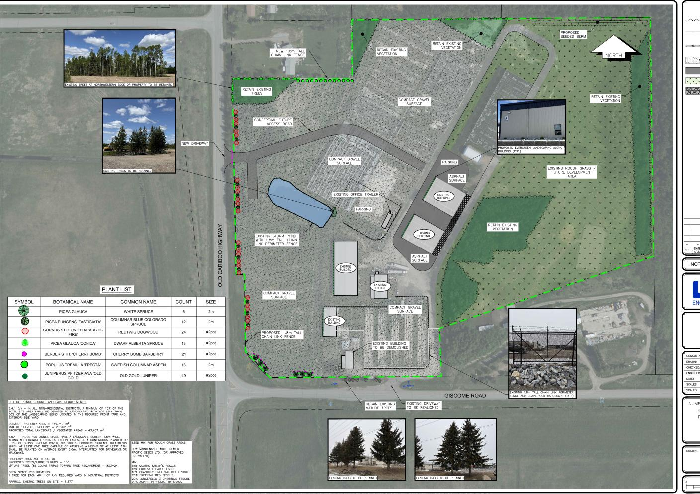
LEGEND (EXACT EXTENT TO BE CONFIRMED ON SITE) EXISTING 1.8m TALL BLACK VINYL COATED CHAIN LINK FENCE PROPOSED 1.8m TALL BLACK VINYL COATED CHAIN LINK FENCE TO MAIN EX. FENCE ALONG GISCOME RD HALT SURFACE
