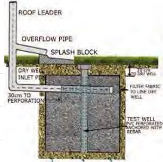
Soak Away Pit
