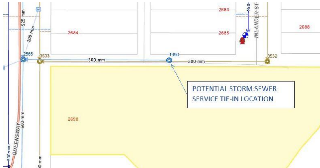
Figure 3: Potential Storm Sewer Service Tie-In Location
