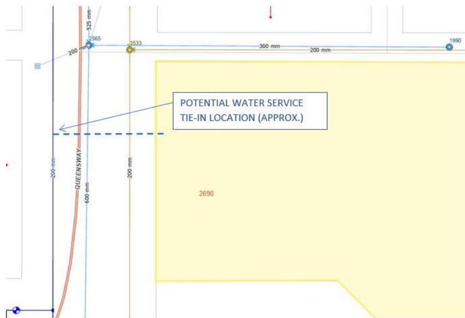
Figure 1: Potential Water Service Tie-In Location
