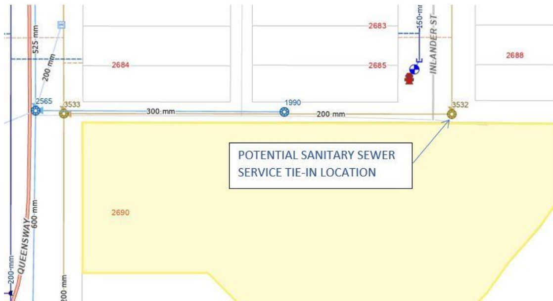
Figure 2: Potential Sanitary Sewer Service Tie-In Location
