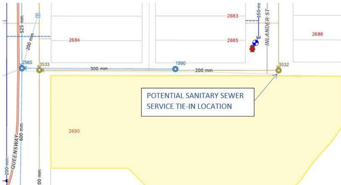
Figure 2: Potential Sanitary Sewer Service Tie-In Location
