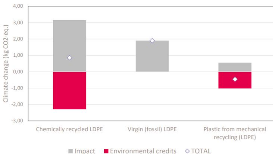
Figure 2 - Plastic Energy LCA and the use of “avoided emissions”
