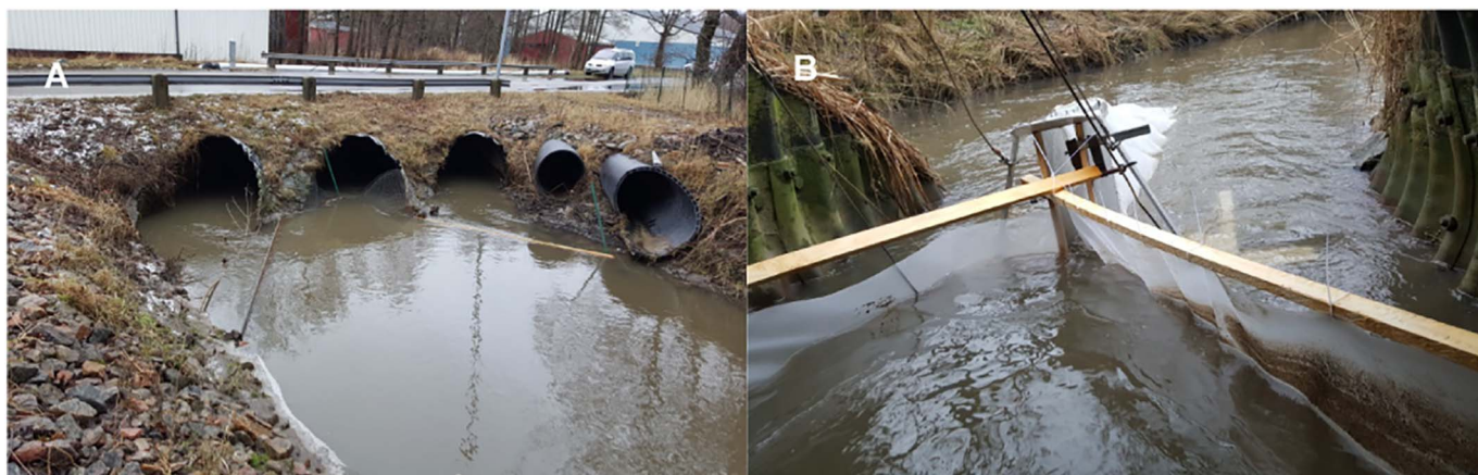
Fig. 2. Sampling setup for measuring the total pellet runoff during 1 h. On the upstream side of the small bridge (A) wooden pieces were placed so to lead the surface water into one of the tunnels and on the downstream part (B) a net was attached which led all the material floating on the surface to a collection sock at the end.
